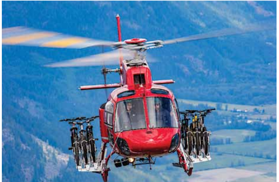
The Quick Release Bicycle Racks allow for up to three bikes to be carried per side, and the manufacturer said the bikes can be removed and installed in less than a minute each.
