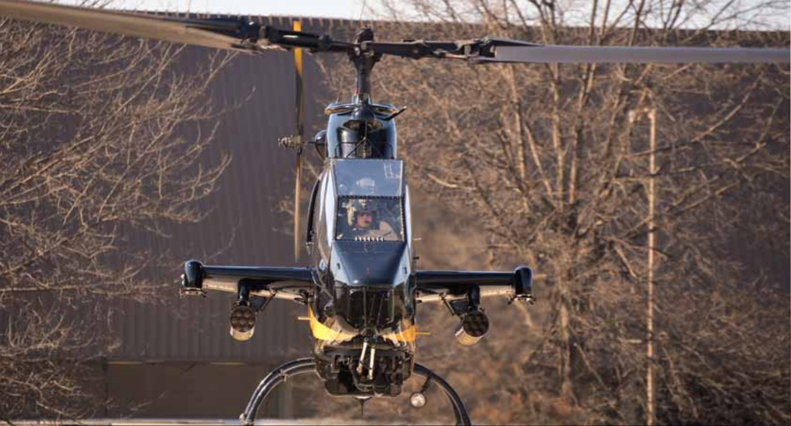
The U.S. Army experienced a number of fatal mast bumping accidents in its Bell AH-1 Cobras and UH-1 Hueys beginning in the 1960s. The Army initially sought to address the problem through pilot education, although Bell eventually designed a hub spring to reduce the risk of mast bumping. Skip Robinson Photo
