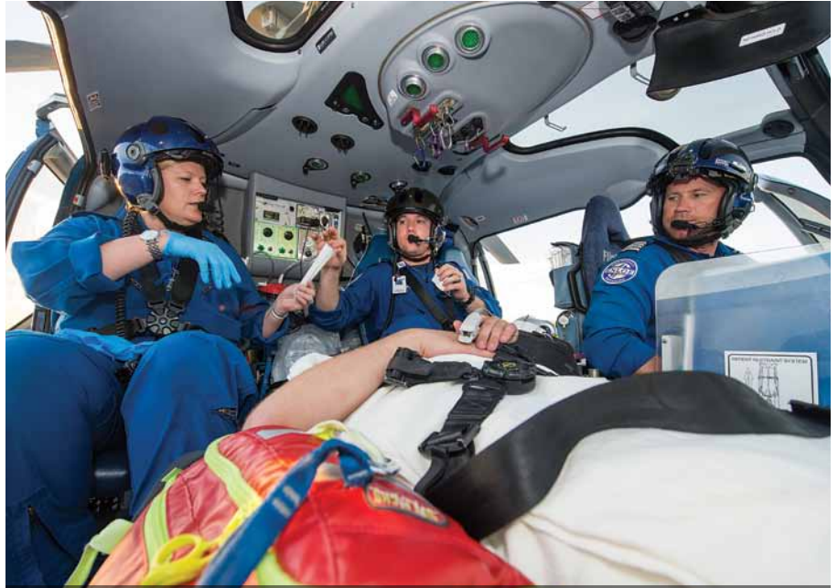
The FlightCare H130's intercom system includes a jack for an electronic stethoscope, allowing nurses and paramedics to listen to blood pressure, lung sounds, or heart tones while in flight.
